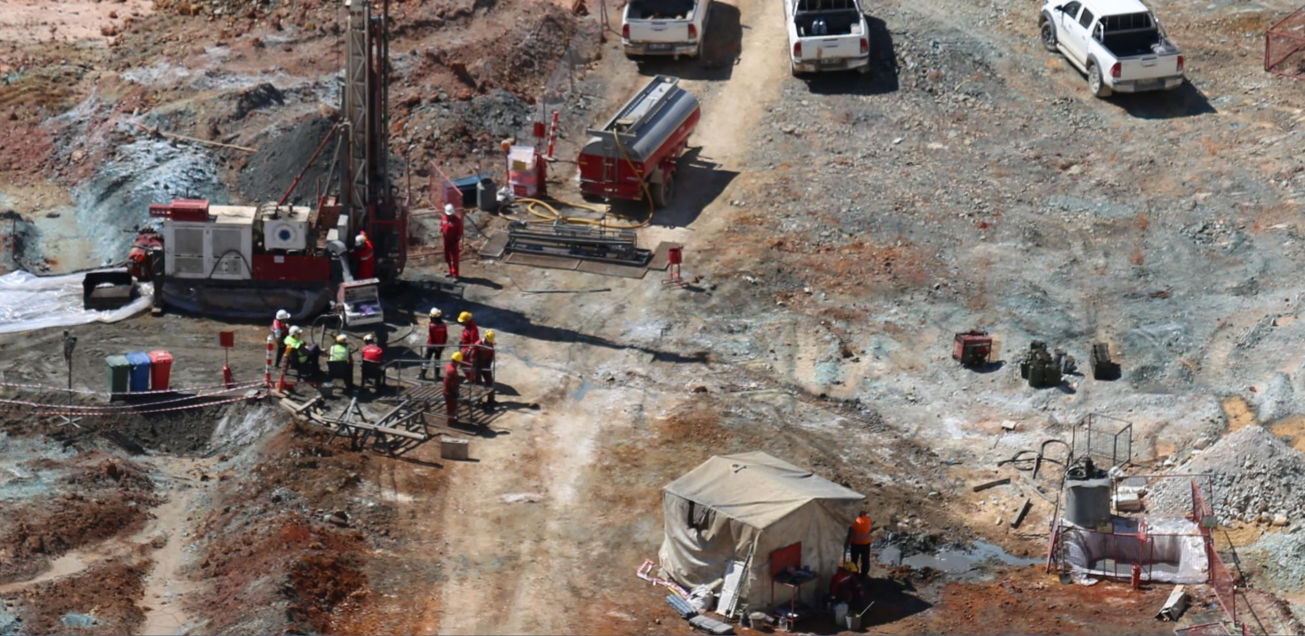
Contractor carrying out infill drilling at Sulphides South Pit
